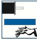
**Do not** use holding torque/detent torque of motor as a fail safe brake.
