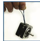
**Do not** hold motor by lead wires.
