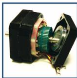
**Do not** disassemble motors; a significant reduction in motor performance will occur.
