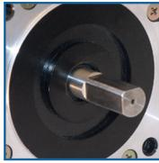
**Do not** machine shafts; this will have a negative effect on shaft run out and perpendicularity.
