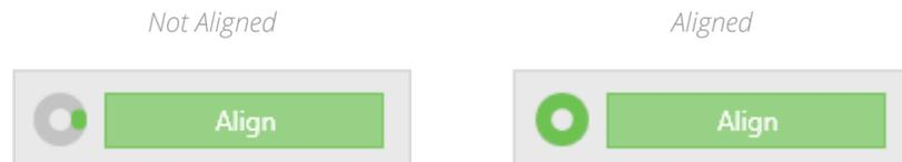
To align an encoder using AMT Viewpoint simply press the “Align” button. This action will only take a second. It is completed when the status circle appears completely green.
