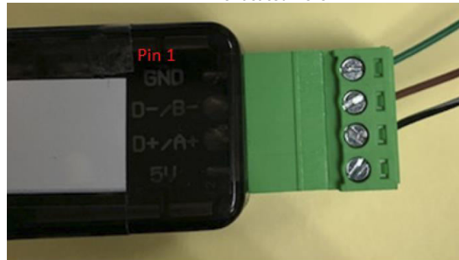
Figure 3: USB to RS485 converter card, p/n USB485
